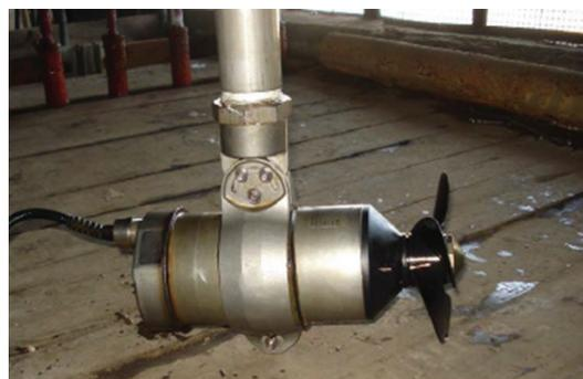
Figure 27: Submersible agitators
